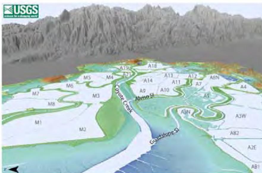
Figure 100. Shaded relief map of full feature LIDAR colored by elevation (vertical exaggeration 5x). Perspective view is looking east towards Coyote Creek. Figure from Foxgrover and Jaffe (2005).
